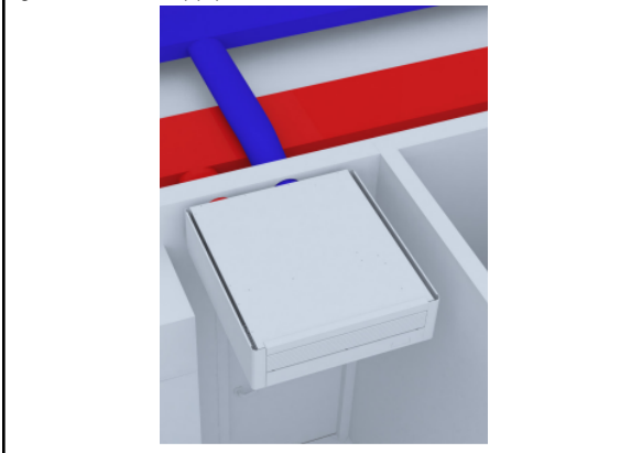
Figure 6. Shared supply and exhaust vents
